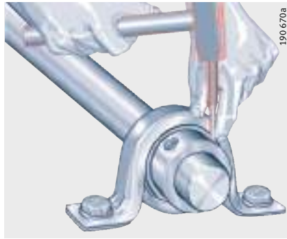
Figure 21 Tensioning the eccentric locking collar
