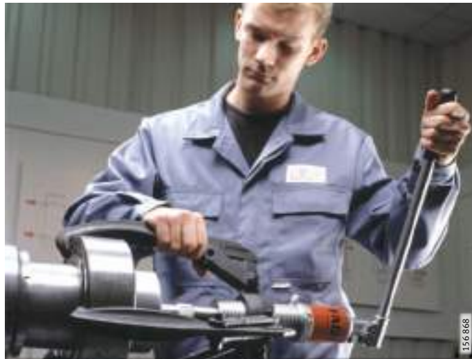
Figure 1 Dismounting of a bearing using a hydraulic extractor
